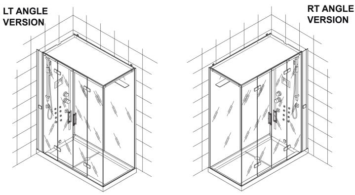
The minimum height of the wall tiles without protrusions is equal to the height of the stall. On the walls there cannot be any greca or quarter round decorative patterns.
